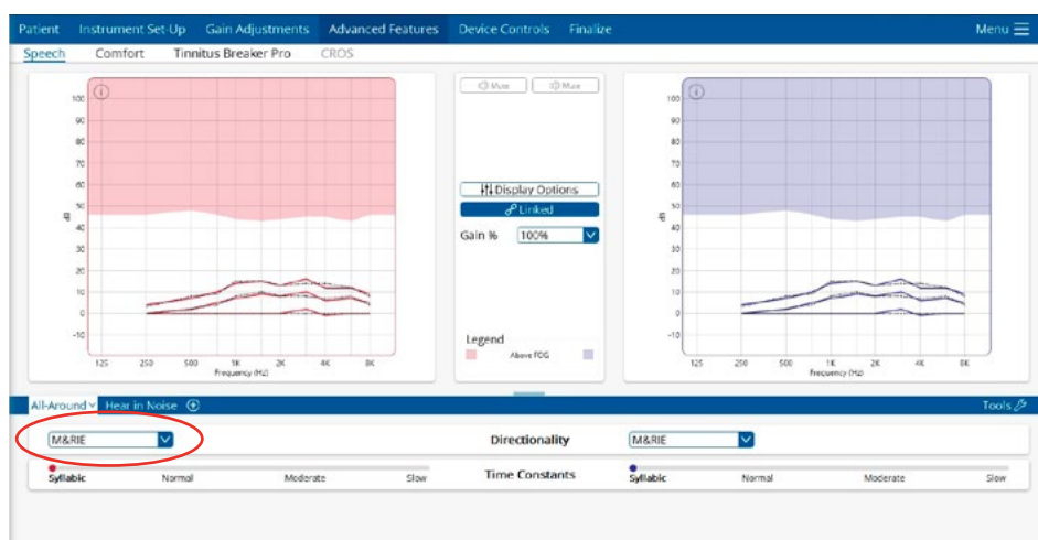
Figure 7. When fit with a M&RIE receiver, the canal microphone is active by default when in CrossLink Directionality 4 or CrossLink Directionality 3. In other programs, "M&RIE" can be selected in the Advanced Features screen.
