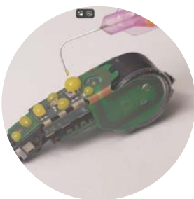
Parylene-coated internal circuitry
