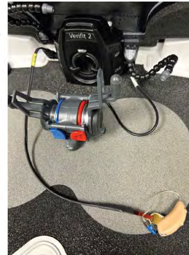
Figure 11 Placement of the battery pill into a hearing aid.
