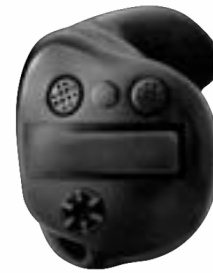
Both Push button and volume control wheel
