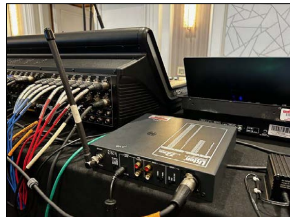
FM System connected to AV system for large conference plenary session
