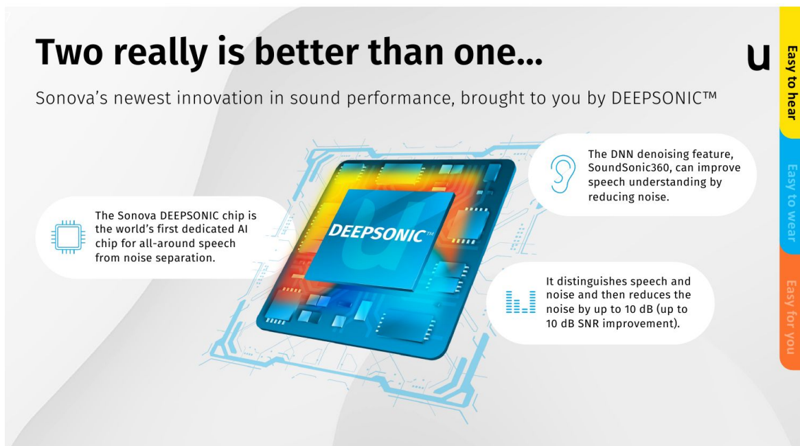
Figure 1. The DEEPSONIC chip separates speech from noise and reduces noise by up to 10 dB.
